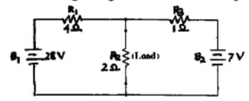
Find out the Current flowing through the Load resistance R<sub>LOAD</sub> using Thevnin's Theorem.
